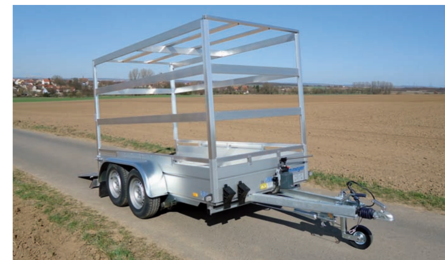
BTSL 2730/151 Zubehör: Reling, Spriegel BTSL 2730/151 Options : main-courante, ossature BTSL 2730/151 Optional extras: top rail, canvas top support
