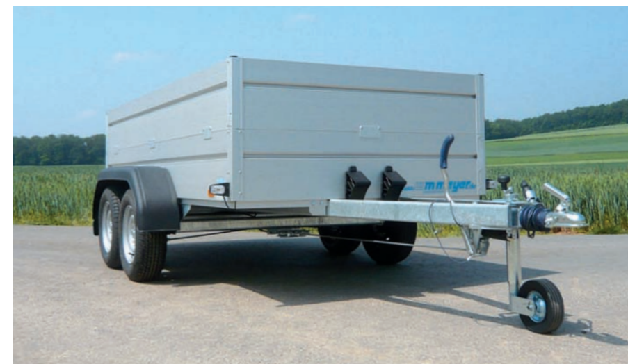
BT 2030/151 Zubehör: Bordwanderhöhung (350 mm) BT 2030/151 Option : ridelles supplémentaires amovibles (350 mm) BT 2030/151 Optional extra: additional panels which can be removed (350 mm)
